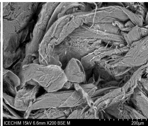
Fig. 4. SEM image of dry cellulose from Cladophora vagabunda sp.
