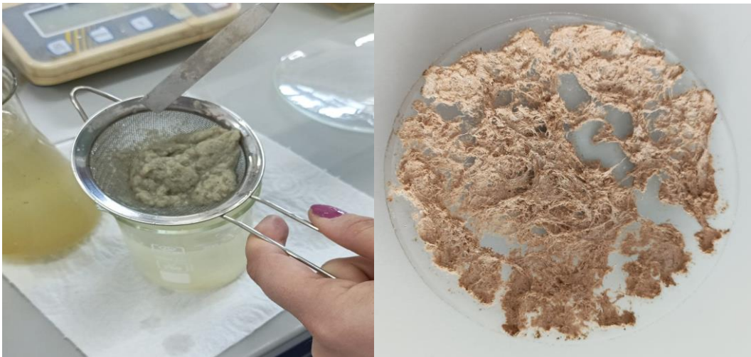
Fig. 2. a) Cellulose washing; b) Dry cellulose from Cladophora Vagabunda sp.
