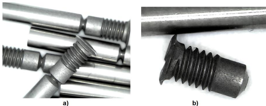
Fig. 1. Samples of the mechanically milled titanium implants with a) (before) anodization) and without b) the suspending rod (after anodization) (2 mm diameter, 4 mm length)
