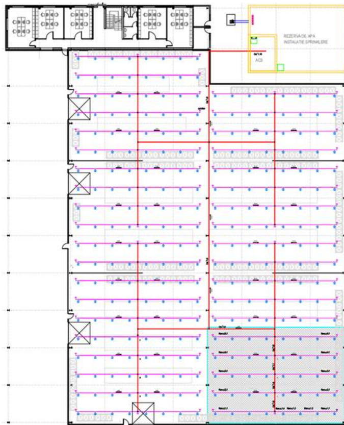
Fig. 3. Sprinklers Positioning and water supplying in the warehouse
