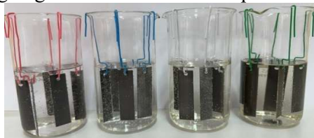
Fig. 1. Experimental set-up for the gravimetric method, at the beginning of the experiment for simple extracts of JR, AS and the mixture of JR + AS
