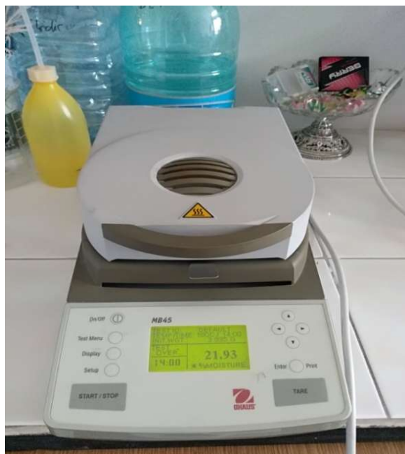
Fig.2. OHAUS thermobalance (moisture analyzer)
